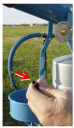
To prevent accidental detonations, bleed remaining fuel by disconnecting rubber tubing from needle valve.
